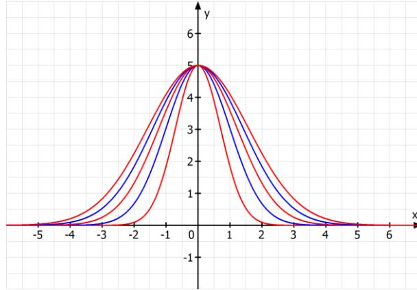
We see the gaussian with variance  $\sqrt{a}$  centered around zero. The smaller  $a$ , the sharper the localization.
