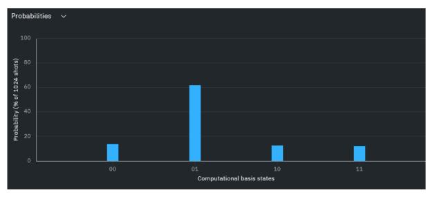
The measurement result with the highest probability is the combination x = 1, y = 0, the solution for our problem. Please note that the composer uses little endian.
