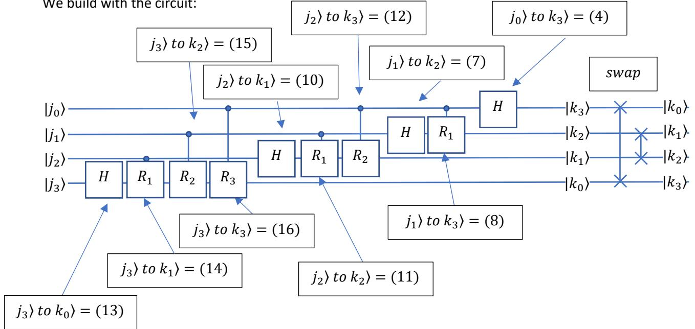
Note: The gates named  $R_1$  and  $R_2$  are the controlled  $S^\dagger$  and  $T^\dagger$  gates. They are special forms of the single qubit unitary rotation gate  $R_k$ :
