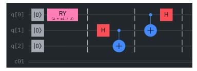
Note: The first Hadamard and CNOT produce the Bell-state  $|\phi^+\rangle$  from qubits  $|A\rangle$  and  $|B\rangle$ .
